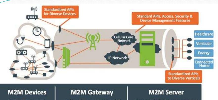
Cellular, WLAN, WPAN (Zigbee, 6LoWPAN, Bluetooth), Wireline Enables cellular & non-cellular M2M devices to communicate through operator networks. Provides localized Service Capabilities to offload network
